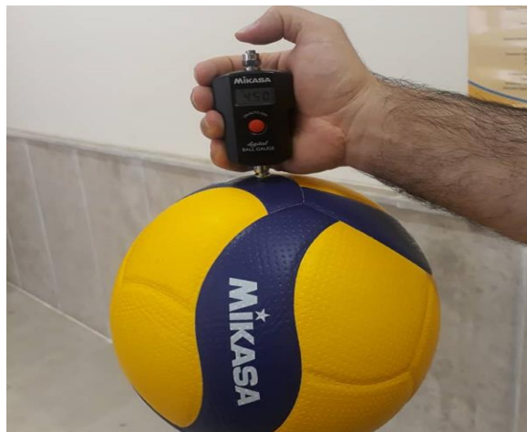
Figure 4- Measuring the air pressure inside samples
