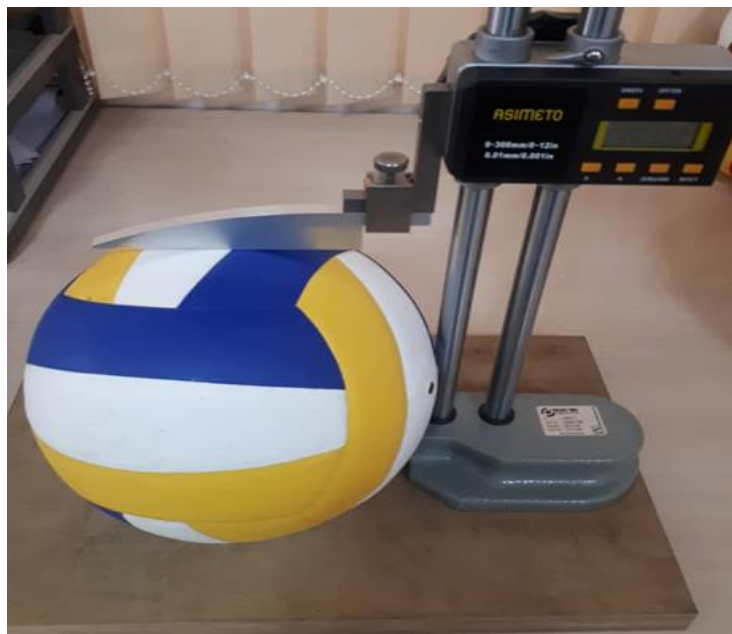
Figure 2- The caliper used to measure the diameter of sample balls
